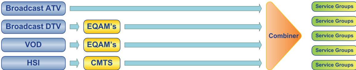
Figure 3: A typical headend using different platforms
